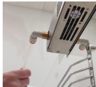
Photos 10, 11: Push 0.25" tubing into the gas fittings on the Smart RH module from the outside and inside of the desiccator.
