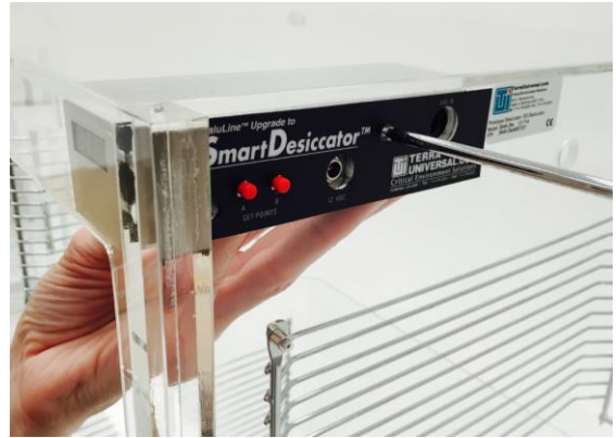
Photos 7, 8: Placing the Smart RH module with gasket and attaching it to the desiccator wall, behind the label
